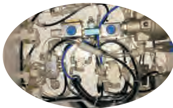
集成气控箱, 内置各种保护/ Integrated gas control box, built-in various protection
